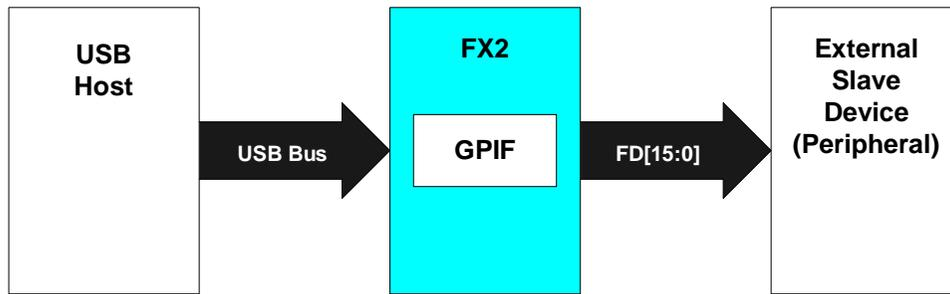
**Figure 1. System Level View of Data Flow in the OUT Direction**
