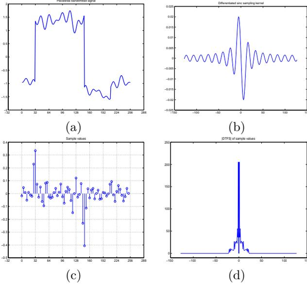
Figure 6: (a) Piecewise bandlimited signal,  $\mathbf{x} = \mathbf{x}_{PP} + \mathbf{x}_B$ , with  $K = 3$ ,  $B = 15$ ,  $R = 0$ ,  $N = 256$ ; (b) Differentiated sinc sampling kernel,  $\psi[n] = d[n] * \varphi_{B+2K(R+1)}[n]$ , bandlimited to  $2K(R+1) + B = 21$  (c) Sample values  $y_s[l] = \langle x[n], \psi[n - lM] \rangle$ ,  $l = 0, \dots, N/M - 1$ ,  $M = 4$ ; (d)  $|DTFS|$  of sample values; Reconstruction error is  $10^{-13}$ .
