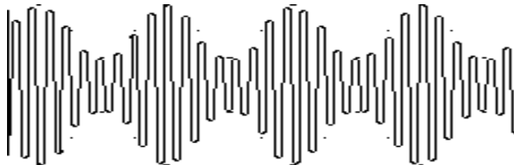
Figure 6 — A carrier signal with modulation
