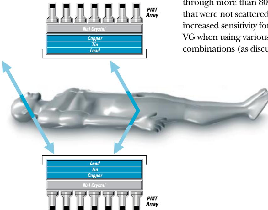
**Figure 7: Millennium VG High Energy Filter Design**
