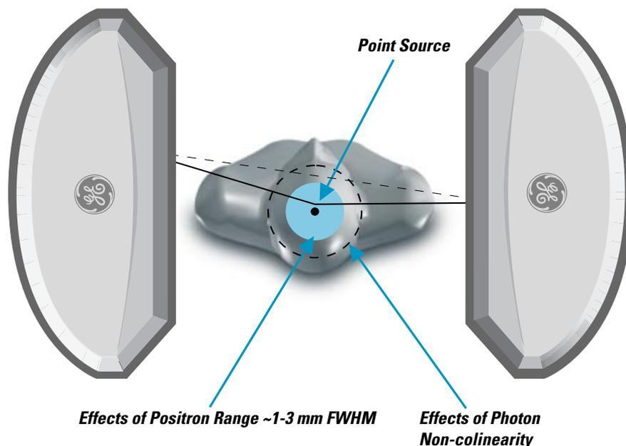
Figure 4: Theoretical Intrinsic Resolution Limits
